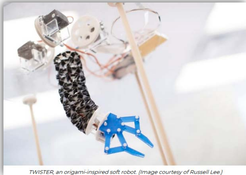
TWISTER, an origami-inspired soft robot. (Image courtesy of Russell Lee.)
